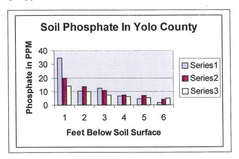
This apparent lack of movement is a function of the insoluble compounds or complexes that are formed by the soil phosphate. As a result of the insolubility of the phosphate the water in the soil (soil solution) doesn't even contain enough phosphate to provide for one day of normal plant growth. Rather, as the plant removes the phosphate from the soil solution, more phosphate can enter the water, which is in turn removed by plants.
